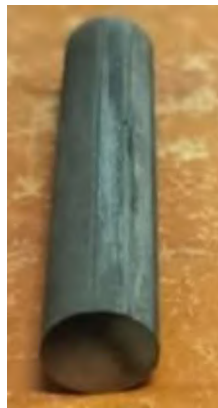
Figure 1. Typical AW-DED component used for tribological study
